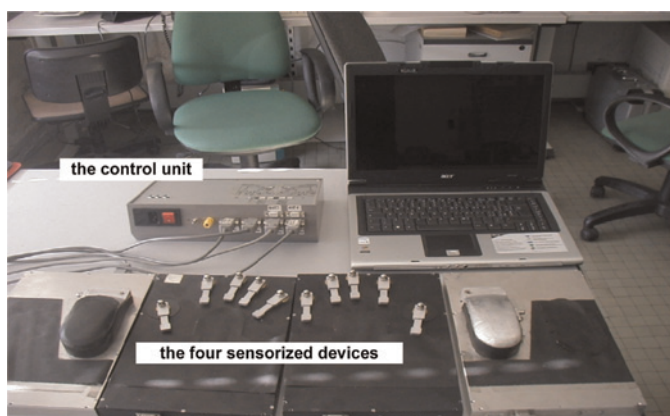
Figure 4 A view of the entire measurement system, including the measurement devices (2 keyboards and 2 mice) and the control unit
